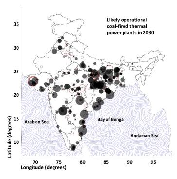
Clusters of coal-fired thermal power plants in 2030. The brown circles represent the thermal power plants operational in 2014 and the second colour represents all the expansions likely to be operational in 2030. The largest circle is 4620MW. Note that many of these circles are overlapping due their close proximity
